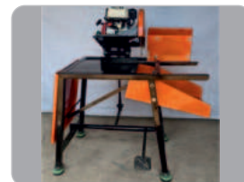
Portable self-propelled cassava sett cutter
