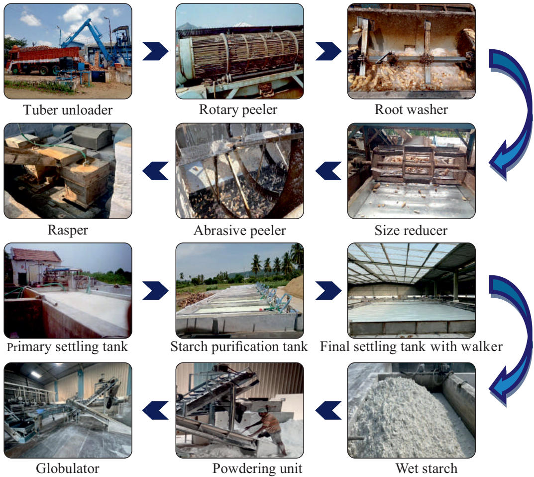
Fig.3. Machineries for the Production of wet starch used for Sago Production
