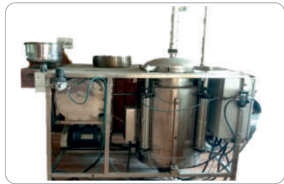
Fig.2 : Vacuum frying system
