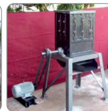
Motorized Output: 300-1100 kg h -1 for chip thickness 2.5-10 mm
