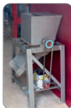
Pedal operated Output: 80-750 kg h -1 for chip thickness 0.9 -6.9 mm
