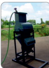
Pedal operated Output: 80-750 kg h -1 for chip thickness 0.9 -6.9 mm
