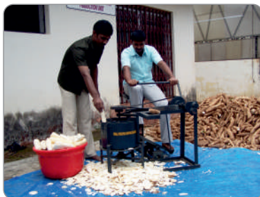
Pedal operated Output: 80-750 kg h -1 for chip thickness 0.9 -6.9 mm
