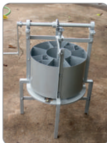
Hand operated Output: 35-120 kg h -1 for chip thickness 2.3-6.9 mm
