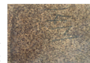
Cassava stem based particle board
