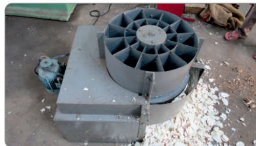
Motorized Output: 300-1100 kg h -1 for chip thickness 2.5-10 mm
