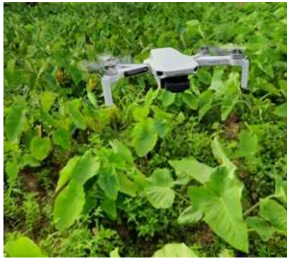
Fig 2. Camera drone collecting aerial images
