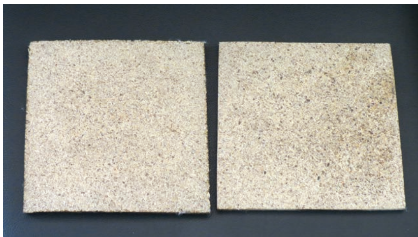
Particle boards from cassava stems
