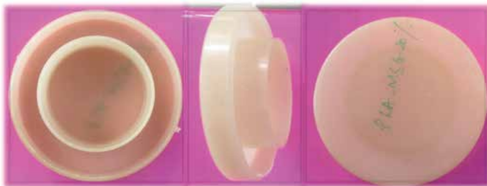
Injection moulded article (jewellery box) with 20% oxidised starch
