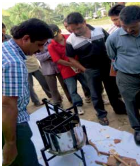
Demonstration of cassava chipping machine
