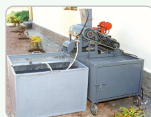
Mobile starch extraction unit
