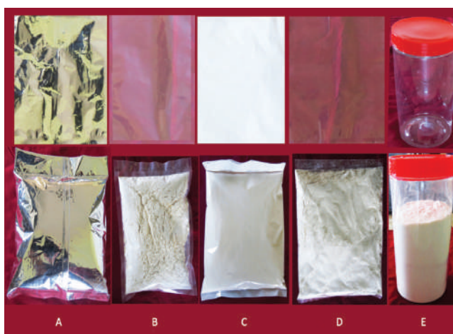
A: Aluminium foil bag B: EVOH bag C: LDPE bag D: PP bag E: PET jar
