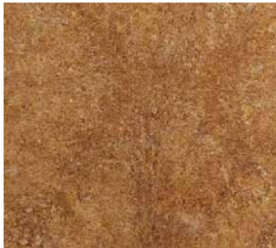
Fig 44. Thermoplastic starch sheet from cassava starch-paddy straw composite flour
