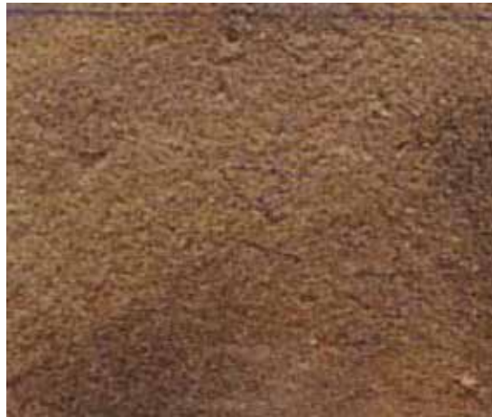
Fig. 43. Thermoplastic starch sheet from cassava starch-rice husk composite flour
