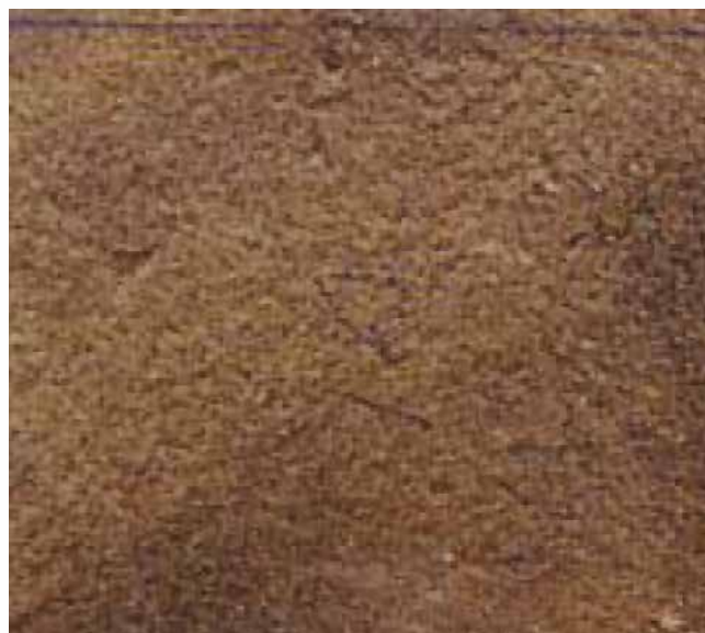
Fig. 123. Thermoplastic starch sheet from cassava starch-rice husk composite flour
