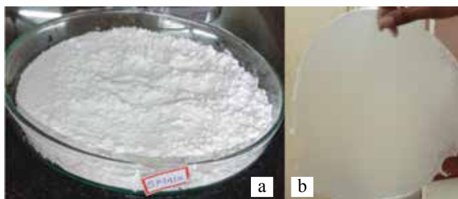
Fig.125. (a) Cassava starch-graft-soybean oil maleate (CS-SOMA) and (b) Biodegradable film prepared from CS-SOMA
