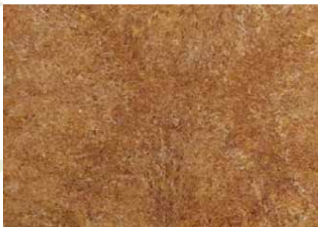
Fig 124. Thermoplastic starch sheet from cassava starch-paddy straw composite flour
