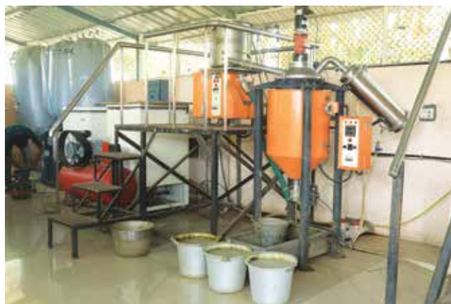
Fig. 146. Apparatus for extraction of biopesticides
