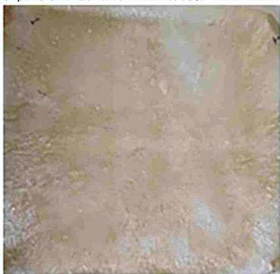
Fig. 76. Thermoplastic starch sheet from cassava starch-stem fibre composite
