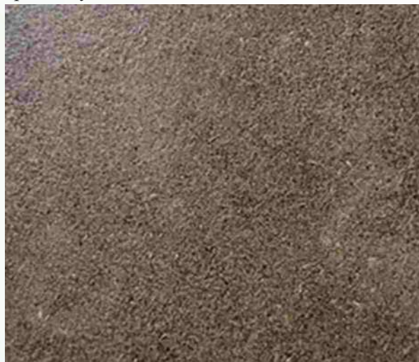
Fig. 74. Cassava stem based particle board
