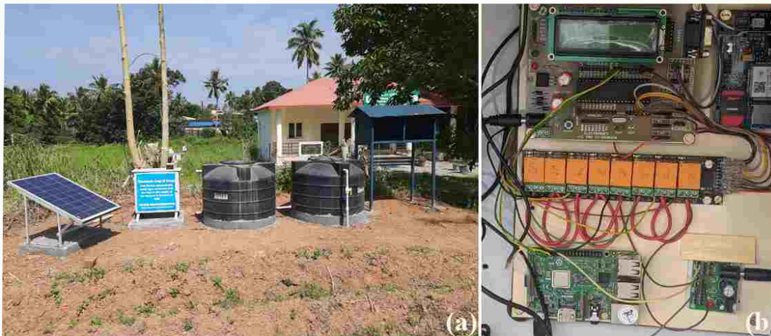
Fig. 92.(a) Smart farming system and (b) Control unit of smart farming system
