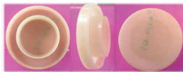
Fig. 43 Injection moulded article (jewellery box) with 20% oxidised starch
