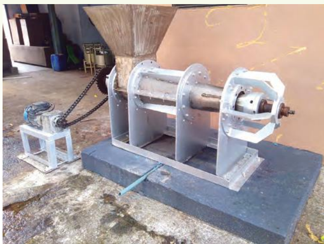
Fig. 79. Continuous screw type pressing machine for dewatering of cassava mash
