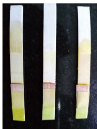
Fig. 117. Validation of DsMV-IgG coated strip (dipstick) developed in ICAR-CTCRI Transgenic Lab. Lane 1 - Strip dipped in DsMV positive control sample leaf sap, Lane 2 - Strip dipped in buffer control sample leaf sap, Lane 3 - Strip dipped in DsMV negative control sample leaf sap, A-Control line, B-Test line
