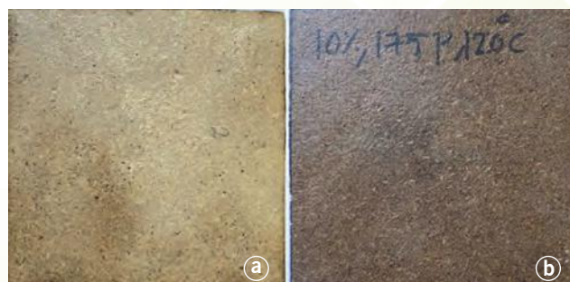
Fig. 80. Cassava stem-based particle boards made using (a) acid modified starch and (b) cashew nutshell liquid as adhesives
