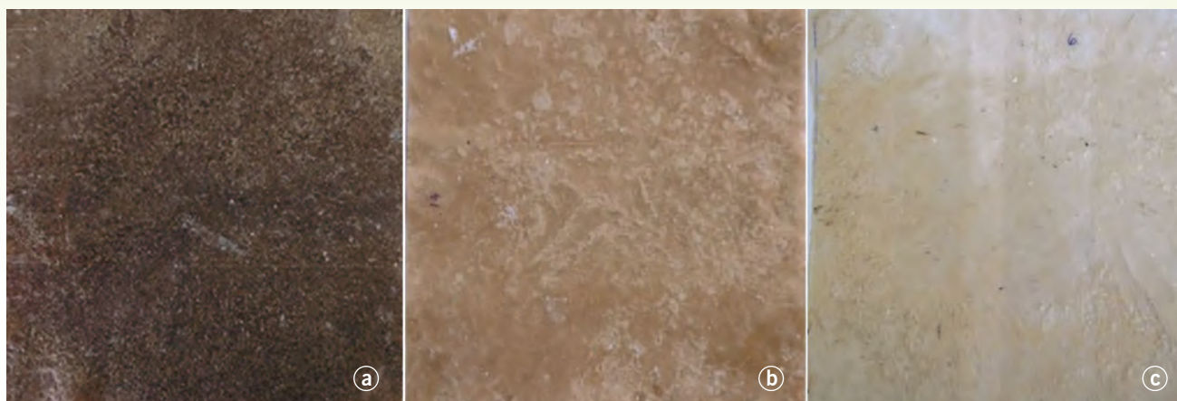
Fig. 82. Thermoplastics starch sheet prepared from (a) cassava starch-saw dust composite, (b) acid modified cassava starch and (c) cassava starch and sorbitol as plasticizer
