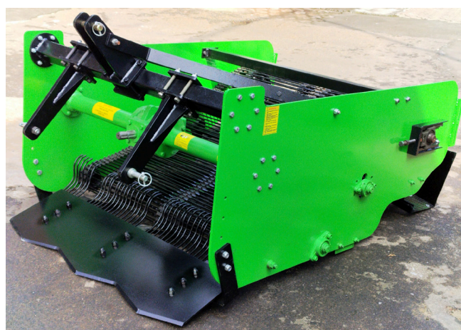
Fig. 51. Tractor operated Chinese potato harvester
