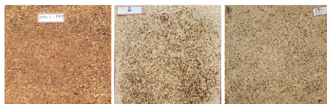
A: Cassava stem-coir pith; B: Cassava stem-rice husk; C: Pretreated cassava stem
