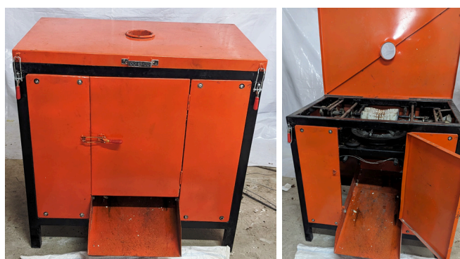
Fig. 69. Continuous type cassava peeler
