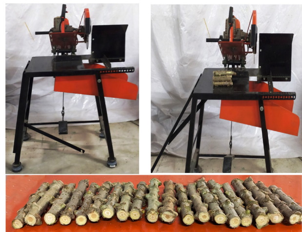
Fig. 52. Portable self propelled tapioca sett cutter
