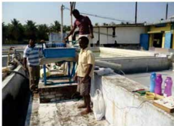
Fig. 53 Industrial evaluation of vibro sieving system at M/S T.A. Perumal Starch Industries, Salem
