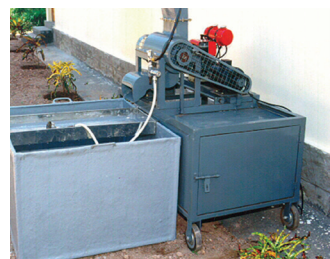
Mobile starch extraction unit Output: 200 kg/h
