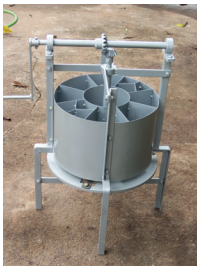
Hand operated Output: 40-120 kg/h for chip thickness 2.3-6.9 mm
