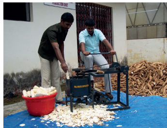
Pedal operated Output: 80-770 kg/h for chip thickness 0.9 -6.9 mm
