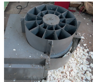
Motorized Output: 290-1100 kg/h for chip thickness 2.5-10 mm
