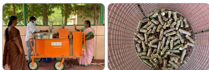
Mobile sugarcane sett treatment device
