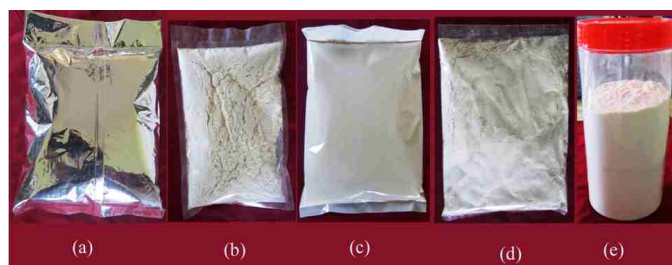
a) Aluminium foil bag b) EVOH bag c) LPE bag d) PP bag e) PET jar Fresh cassava flour stored in different packaging materials
